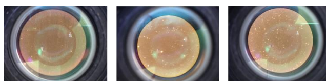
Figure 1. Optical images of the prepared films (magnification ×70): a) Pure gelatin film (left), Gelatin-Glycerol film (middle) and Gelatin-Glycerol-Tea (right)
